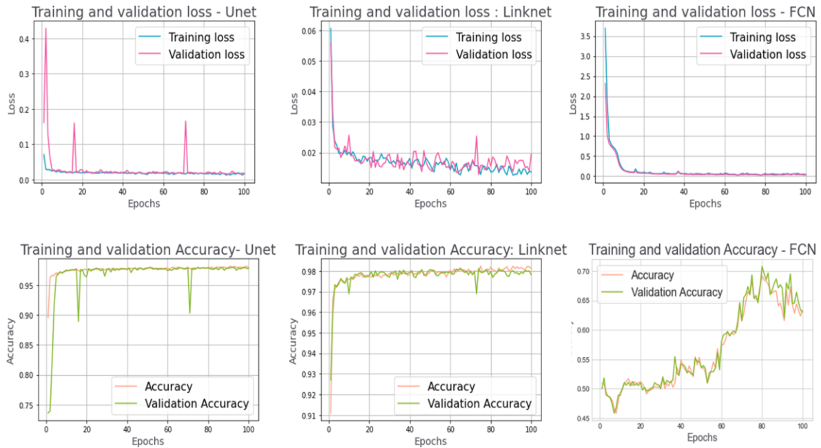
Fig. 6: Training and validation accuracies and losses for LinkNet, U-Net, and FCN8 neural networks
