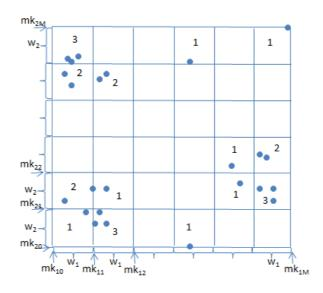
Fig.4: An illustration of dividing a dataset having D=2 into a set of cells.
