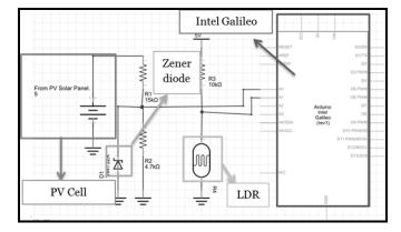
Fig. 3: Sensor Node Circuit Connection
