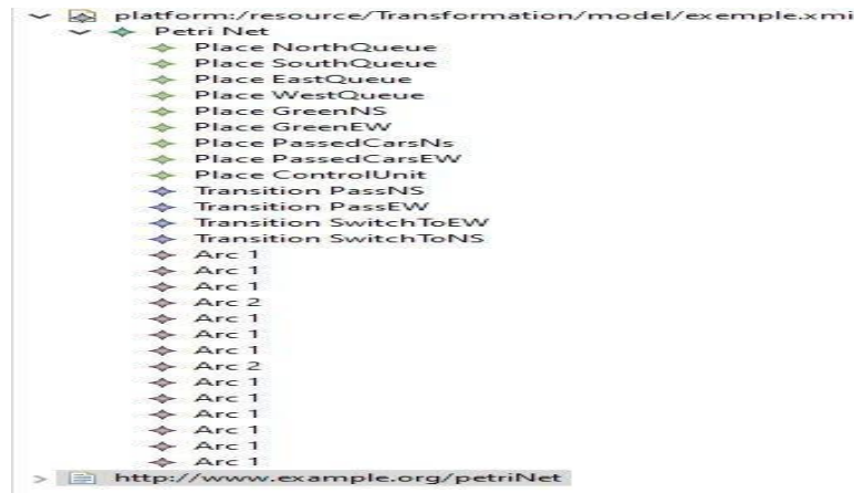
Fig 12: Smart Traffic Management System modeled as a Petri Net
