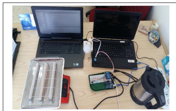
Figure 6. Turn the ceramic heater on when receiving the voice command “Heater on” (see the red bar in the middle)
